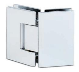
• Glass thickness 8, 10, 12 mm · Self-closing from 15° · Continuously adjustable zero position · For mounting doors to a fixed sidelight
