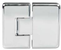
• Glass thickness 8, 10, 12 mm · Self-closing from 15° · Continuously adjustable zero position · For mounting doors to a fixed sidelight
