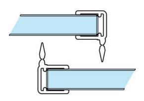
$\mbox{\Large 1}$  Glass thickness 8 mm  $\cdot$  sealing strips between fixed sidelight and sliding door  $\cdot$  Packaging unit 1 pair
