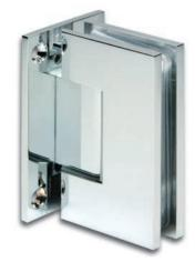
$\bigcirc$  Glass thickness 8, 10, 12 mm  $\cdot$  Self-closing from 15°  $\cdot$  Continuously adjustable zero position  $\cdot$  Supplied without mounting hardware
